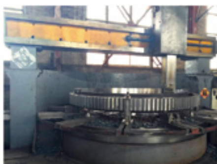
4m 数控立车 4m CNC Vertical Lathe
