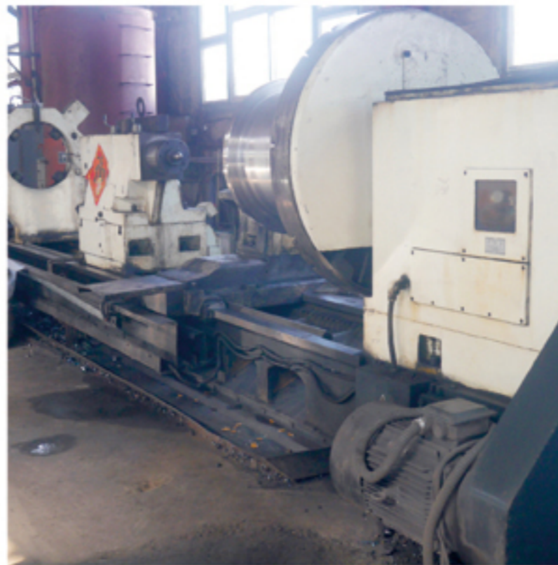
1.8m数控卧车 1.8m Horizontal Lathe
