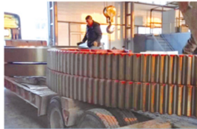
齿圈轮带/ Girth Gear Tyre \Phi=5.4m
