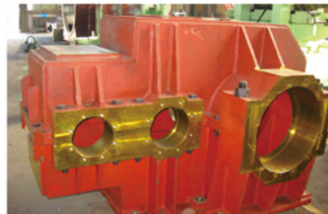
减速机箱体/ Gear Reducer Box H=1.8m L=3m
