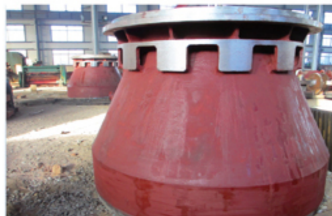
回转窑出料口/ Outlet of Rotary Kiln
