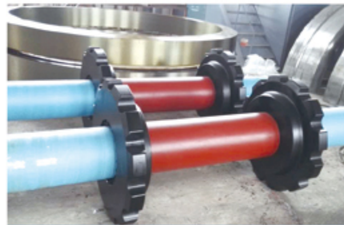
链轮/ Chain Wheel \Phi=1.1m
