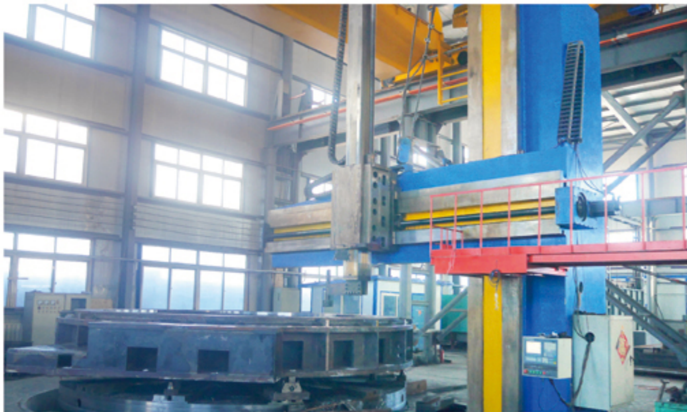
14m数控立车 14m CNC Vertical Lathe
