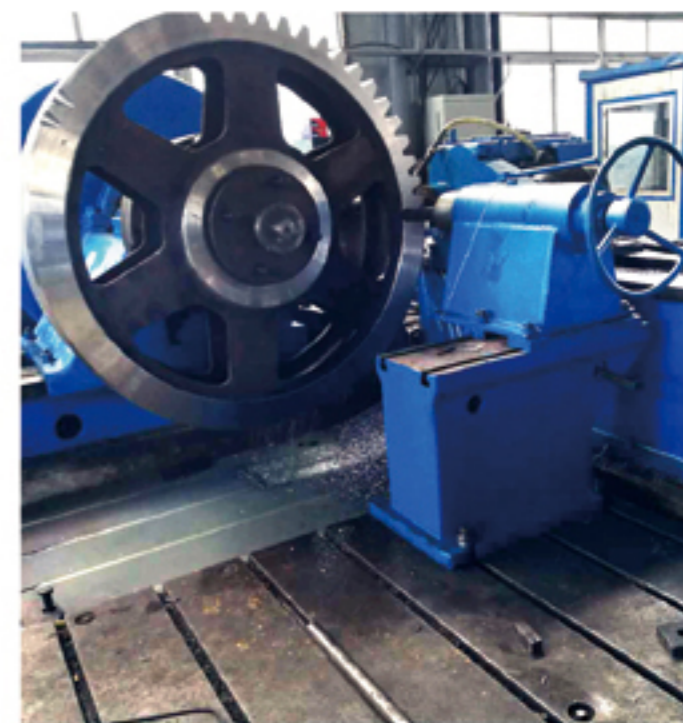
5米人字铣 5m Double Helical Gear Milling Machine
